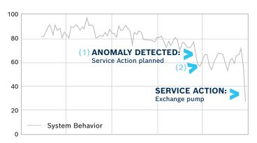
Minimal production restrictions: After a cavitation was predicted, a pump was replaced at the weekend as planned.
