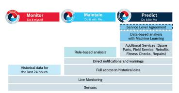
▲ CytroConnect Solutions: three tiered service packages to prevent downtimes – from real-time monitoring alone to a "flat rate" with spare parts management.
