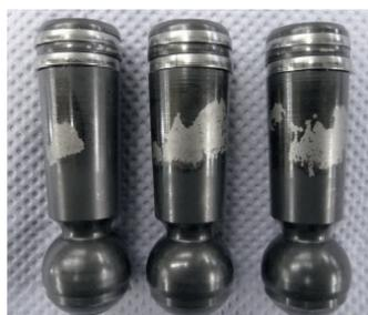
▲ **02 Fluid-related damage to various components of an axial piston pump.**
