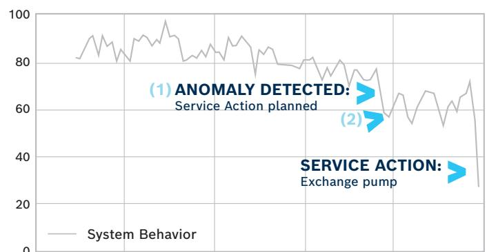
▲ **Minimal production restrictions:** After a cavitation was predicted, a pump was replaced at the weekend as planned.
