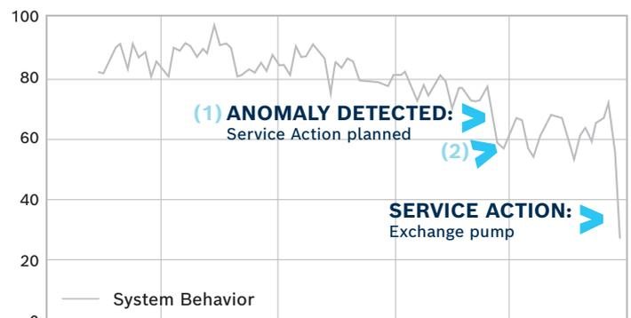
▲ **Minimal production restrictions: After a cavitation was predicted, a pump was replaced at the weekend as planned.**
