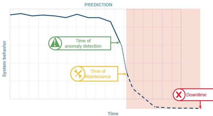
▲ Example from a recycling system: After anomalies were detected (1) and maintenance recommendations were given, the operator has one week in which to rectify the fault.
