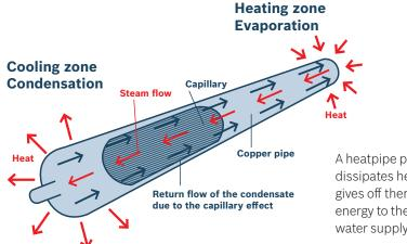
A heatpipe passively dissipates heat and gives off thermal energy to the cooling water supply.
