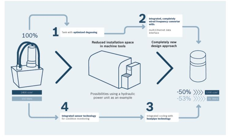
Evolution compact: With four key innovations integrated hydraulic aggregates gaining installation space.
