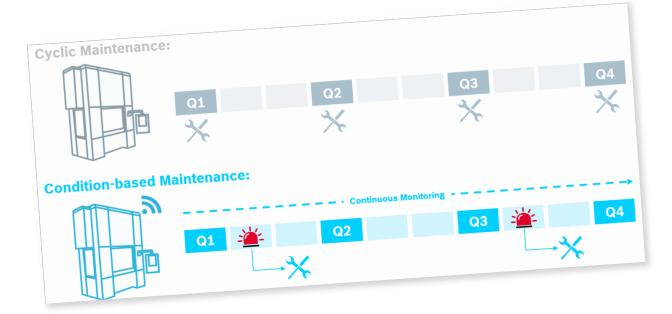
▲ 02 Cyclic maintenance versus condition-based maintenance by means of Predictive Analytics
