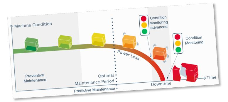
▲ 01 Predictive maintenance uses locally collected data and cloud analyses to calculate the optimal service intervals.
