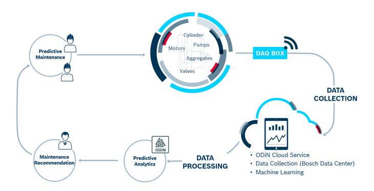
▲ 02 From the local data collection to the cloud-based analysis: the individual components of predictive maintenance as a service.
